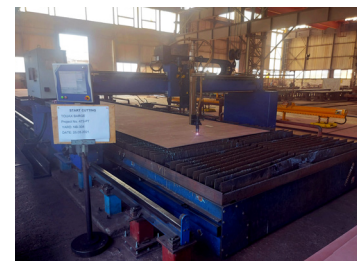
Plasma cutting of the first steel plate
