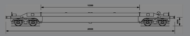
These wagons were built in 1998 in Finland and are approved for UK domestic traffic only. The pocket wagon feature of these wagons has been designed to accommodate either  $2 \times 20^\circ$  or  $1 \times 40^\circ$  containers up to  $9^\circ6^\circ$  high within the UK domestic structure gauge.
